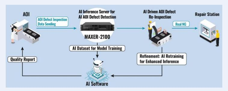
These algorithms leveraged deep learning through approximately 30 photographs per component at an inference rate of 0.03s, with which a baseline was established to assess components against. The acceleration provided by the installation of additional GPUs in the <a href="MAXER-2100">MAXER-2100</a> worked to enhance the efficiency of these AI algorithms, shortening the time needed to detect defects to just 0.05s per photograph.
